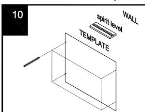
Please use the template provided to mark on the wall the position of the fixing.
