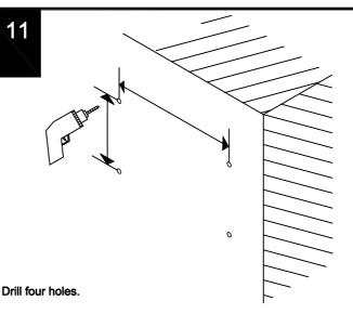
Warning: Always ensure wall area to be drilled is free from hidden electrical wires, water and gas pipes.
