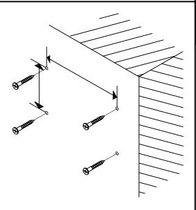
Insert an appropriate wall plug into each hole.
