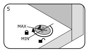
The panels are locked when each cam is turned to between 1/2 and 2/3 of a full turn (Maximum rotation)
