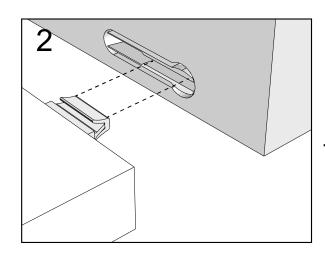
Push connector into housing to join.
