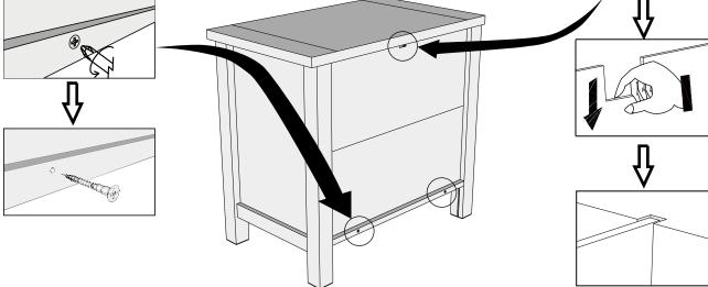
Step2: Press down all the back panel so it is clear of the top panel slot;
