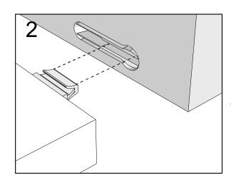
Push connector into housing to join.
