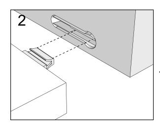
Push connector into housing to join.
