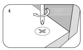
Use a cross-point s crewdriver (PH2 or P Z2 is ideal) to tighten the cams and lock the panels together.
