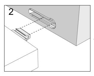
Push connector into housing to be jointed.
