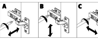
A. Side to side adjustment by clockwise or anticlockwise adjustment.
