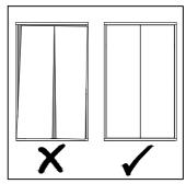
Please ensure all doors are aligned and evenly spaced before applying the back panel fixings.
