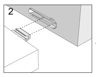
Push connector into housing to join.
