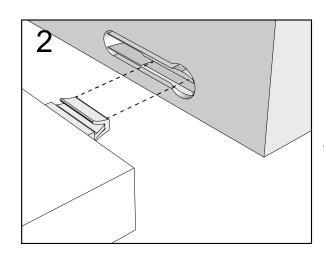
Push connector into housing to join.
