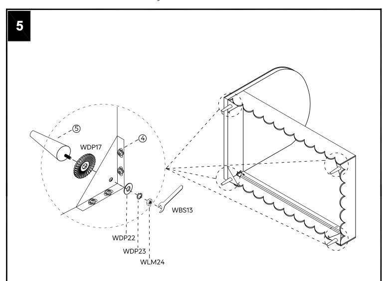
Fully tighten all the bolts at this stage.
