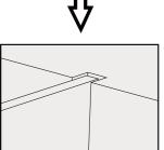
Step2: Press down the two back panels so they are clear of the top panel slot;
