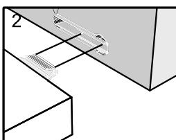
Push connector into housing to be jointed
