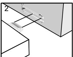
Push connector into housing to be jointed
