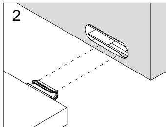
**Push connector into housing to be jointed.**
