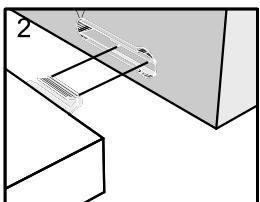
Push connector into housing to be jointed
