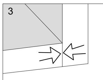
**Push connector into housing to be jointed.**
