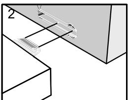
Push connector into housing to be jointed
