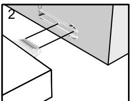
Push connector into housing to be jointed
