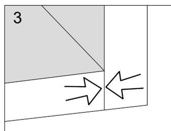
**Push connector into housing to be jointed.**
