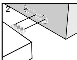
Push connector into housing to be jointed
