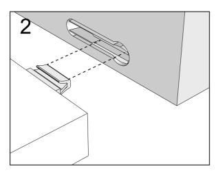
Push connector into housing to be jointed.
