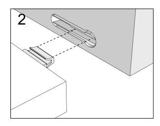
Push connector into housing to be jointed.
