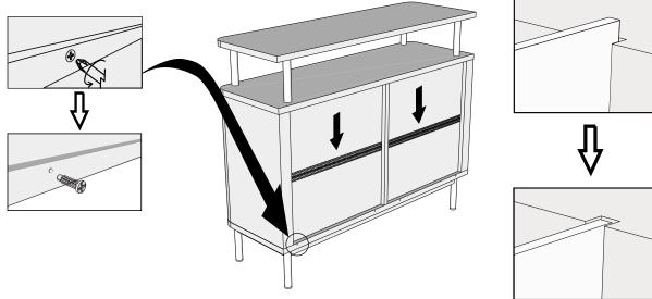
Step2: Press down the two back panels so they are clear of the top panel slot;
