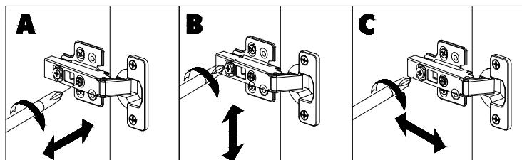
A. Side to side adjustment by clockwise or anticlockwise adjustment .
