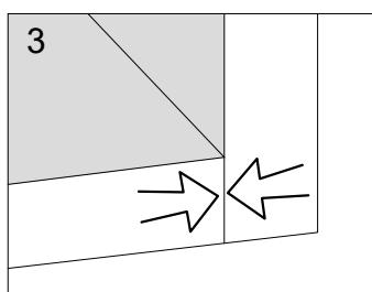
**Push connector into housing to be jointed.**
