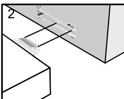
Push connector into housing to be jointed
