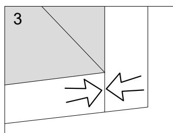
**Push connector into housing to be jointed.**
