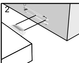
Push connector into housing to be jointed
