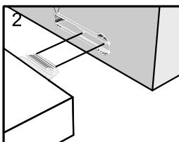
Push connector into housing to be jointed
