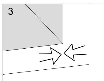
**Push connector into housing to be jointed.**
