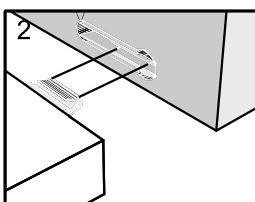
Push connector into housing to be jointed
