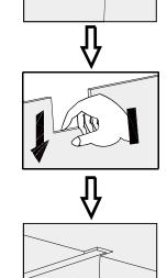
Slide the top panel front to unlock, then lift off. Follow the same sequence to remove the other panels;
