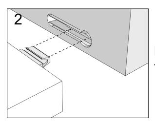
Push connector into housing to be jointed.
