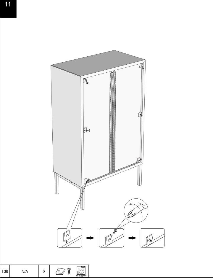
We recommend the use of the wall attachment bracket/strap provided for safety reasons. Secure the strap to the wall with an appropriate screw and wall plug for your wall type (not provided). To hide the strap behind the unit ,drill the hole lower than the top of unit.
