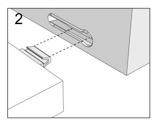
Push connector into housing to be jointed.
