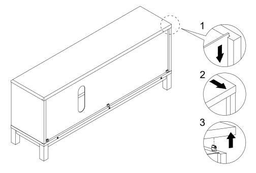
Press the back panels downward so that the top panel can be slide off.
