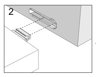
Push connector into housing to join.
