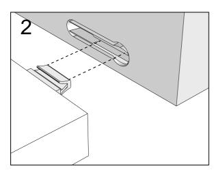
Push connector into housing to be jointed.
