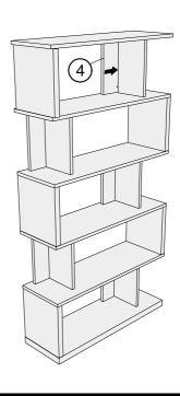
Slide the top panel front to unlock, then lift off. Follow the same sequence to remove the other panels.
