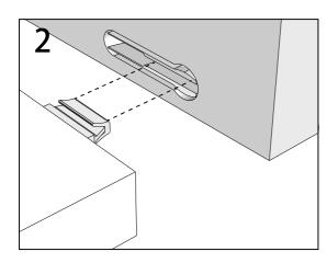
Push connector into housing to be jointed.
