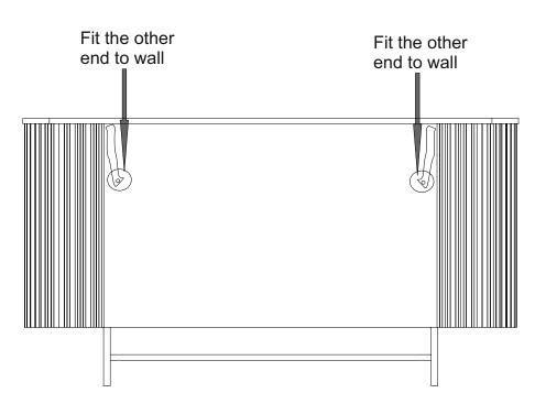
Note: Fit the other end of anti-tip straps provided on both top corners of the rear side of the product to wall
