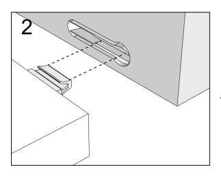
Push connector into housing to join.
