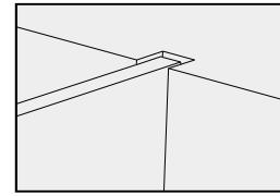
Step2: Press down the back panels so they are clear of the top panel slot;
