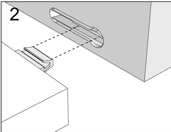
Push connector into housing to be jointed.
