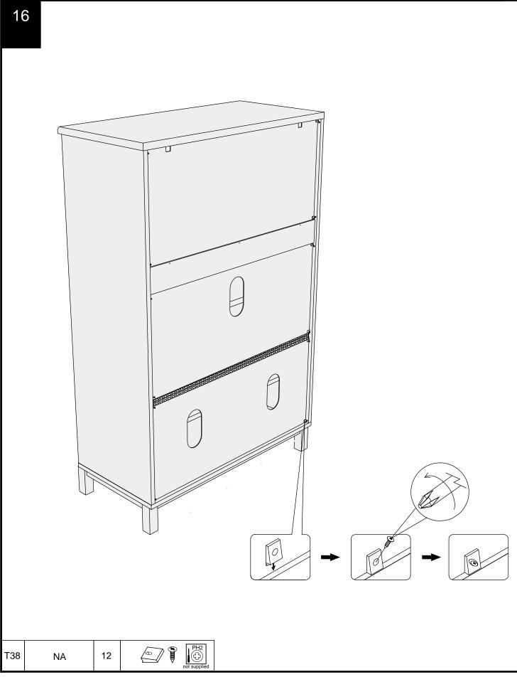
17 We recommend the use of the wall attachment bracket/strap provided for safety reasons. Move unit into desired position.Secure the 2X"L" metal brackets to the wall with an appropriate screw and wall plug for your wall type (not provided).
