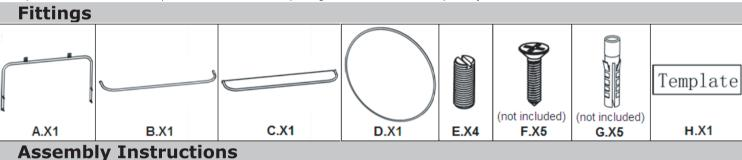
Step 1. Secure the rail (B) and shelf (C) to frame (A) by tighten 4pcs screws (E) with a mini screwdriver.
