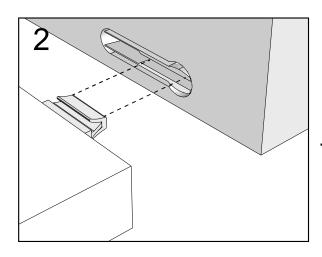
Push connector into housing to join.
