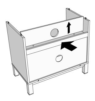
Step5: Lift the back panel (5) up, then slide the side panel (4) and side panel (8) front to unlock, then lift off.
