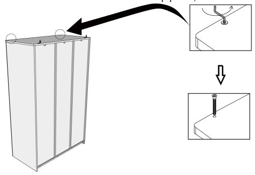
26 Remove the screws from the rear of the panel(2); Step2:
