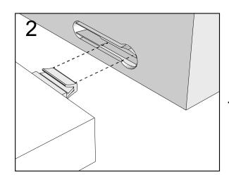
Push connector into housing to join.
