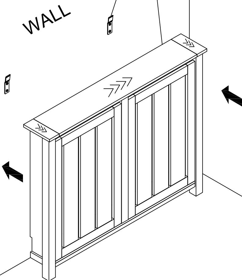
1. Hang the unit to the metal bracket as shown.
