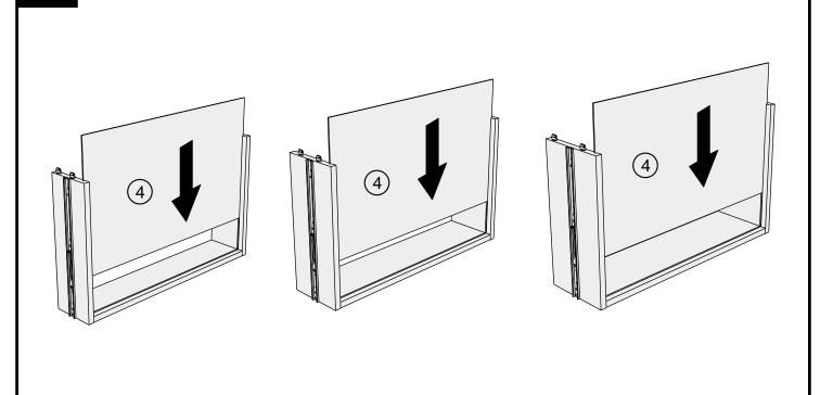
Note: Drawer will be permanently assembled once panel 5 and panel 9 and panel 13 are fitted.
