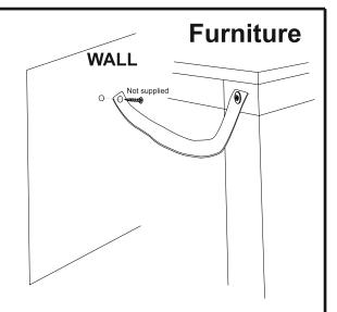
Note: Fit the other end of anti-tip straps provided on both top corners of the rear side of the product to wall
